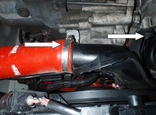
6. Remove the MAP sensor and install the boost take off block using the long screws supplied. Please note the cork casket is between the pipe and the block, the boost take off is also closest to the plastic pipe as shown below.
