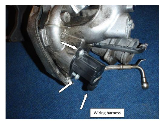
2. Fit the blanking plate to the turbo using the original dump valve torx bolts.
