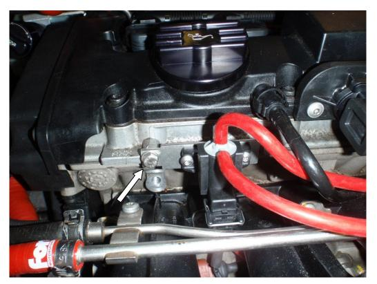
5. Remove the Plastic boost pipe by removing the hose clamps the 10mm nut and the T30 torx that secures the pipe to the engine block this can be tricky due to limited space.
