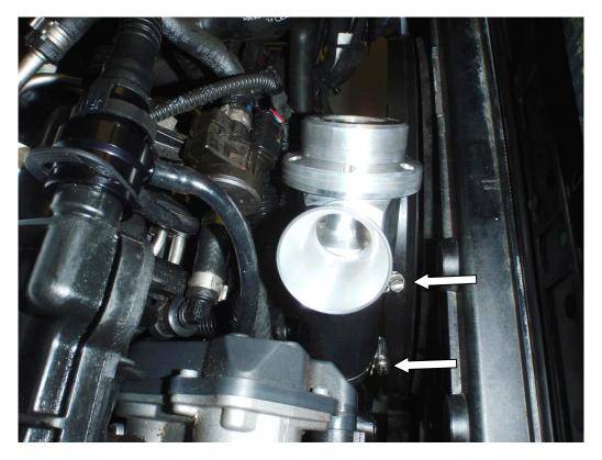
9. The photo below shows how to install the vacuum hoses and wiring extension. When installing in the car, the vacuum hoses and wiring extension can be routed under the inlet manifold for a neat installation.
