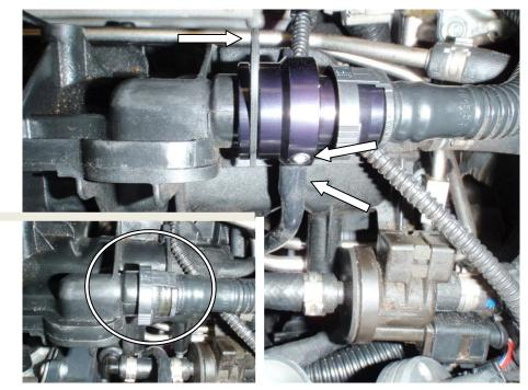
4. Using the bracket Supplied install the solenoid/bracket as shown below. You will need to plug the supplied wiring harness into the OEM Diverter valve wiring harness to do this you will need to reroute the wiring alongside the cam belt cover.
