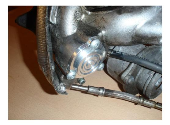
3. Unclip the breather and install the PCV take off, the take off should have two of the holes blocked off with grub screws unless you wish to fit a boost gauge etc. The other hole needs a vacuum take off with the largest hole screwed in. Secure the PCV take off with the small plastic clip supplied in the kit.
