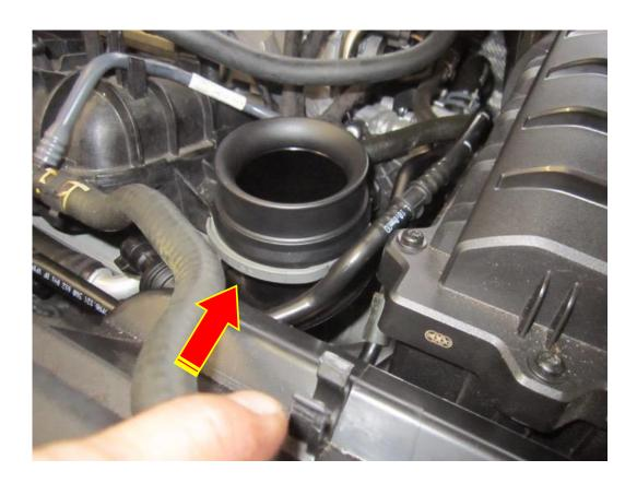
7. Fit the supplied O ring into the machined slot of the smaller two-piece Forge coupler as shown in the picture below.
